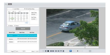
Before you search the SD record, you should trigger the SD recording in motion detection alarm or alarm input alarm (see Motion Detection Trigger or Alarm Input Trigger for detail information).
