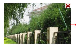
The camera's angle of depression is not wide enough; there are so many trees in the scene. The above mentioned environment is too complex to detect the intrusion
