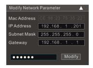
For example, the IP address of your computer is 192.168.1.4. So the IP address of the camera shall be changed to 192.168.1.X. After modification, please input the password of the administrator and click "Modify" button to modify the setting.
