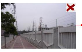
The camera's angle of depression is not wide enough; the street lamps at night lead to light interference; the swaying trees in a windy day lead to random interference. All the above mentioned factors make the scene improper for intrusion detection.
