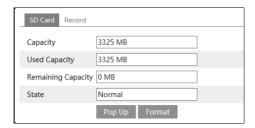
The first time you use the SD card, you should click "Format" button to format the SD card. Click "Pop Up" button to stop writing data to SD card. Then the SD card can be ejected safely.
