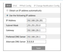
**Use IP address (take IPv4 for example)-**There are two options for IP setup: obtain an IP address automatically by DHCP protocol and use the following IP address. Please choose one of the options for your requirements.
