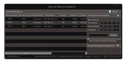
③ Modify the IP address. The default IP address of this camera is 192.168.226.201. Click the information of the camera listed in the above table to show the network information on the right hand. Modify the IP address and gateway of the camera and make sure its network address is in the same local network segment as that of the computer. Please modify the IP address of your device according to the practical situation.
