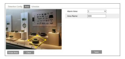
Set the alarm area number and then input the alarm area name. You can add 4 alarm areas at most.
