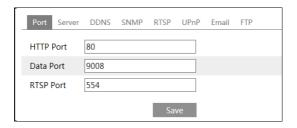
**HTTP Port**: The default HTTP port is 80. It can be changed to any port which is not occupied.
