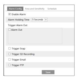
1. Check "Enable Alarm" check box to activate motion based alarm, choose alarm holding time and set alarm trigger options.
