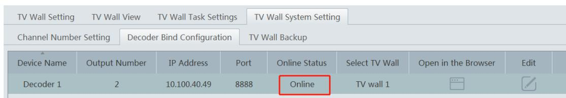
Return to the decoder management interface as shown above. The online status of the decoder indicates that the decoder is successfully bound with TV wall. Go to TV Wall Setting interface as shown below. Drag the outputs of
