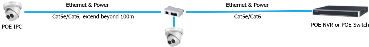
POE Extenders Cascade Deployment , powering 3 IP cameras over one Cat5E cable
