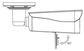
♦ Loosen the screw on the OSD panel, Open the OSD panel, Adjust OSD joystick on the panel.
