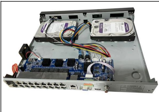
Figure 1-3-3 Connect the power and data cables
