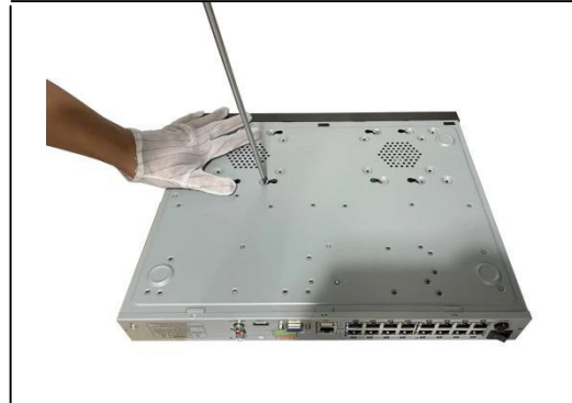
Figure 1-3-2 Fix the HDD
