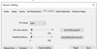
Figure 5-6 FFC control interface
