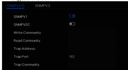
Step 3 Input the parameters of protocol.
