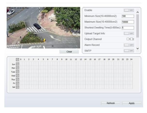
Step 2 Set all parameters for object left. Table 4-7 describes the specific parameters.
