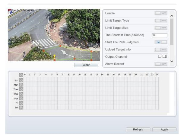
Step 2 Set all parameters for loitering. Table 4-5 describes the specific parameters.
