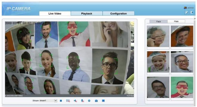
Click "AI" icon to enter AI multiobject interface, as shown in Figure 2-10. The upper right of interface can switch face snapshot and license plate snapshot.
