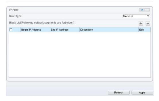
Step 2 Click the button on to enable IP Filter.
