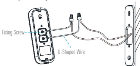
**Option B** Connect the fuse wire with your existing doorbell wire.
