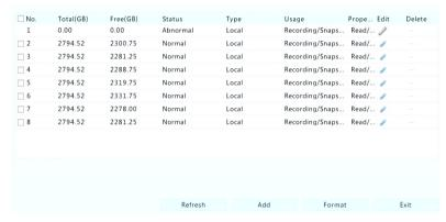
To add a disk, click Add. In the dialog box displayed, select disk usage (recording/snapshot or backup) and disk type (currently NAS only), enter the server address and directory, and then click **Add**. Up to eight NAS disks are allowed.
