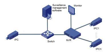
The NVR, IP cameras, and PC are connected on a private network (or LAN). The IP cameras can be connected to the NVR directly or via a switch. The PC is installed with surveillance management software. You can manage the NVR and the connected IP cameras using the surveillance software or through the monitor.
