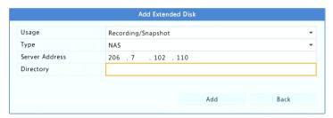
To edit disk property, click , and then modify disk usage (recording/snapshot or backup) and disk property (Read/Write, Read Only or Redundant) as needed.
